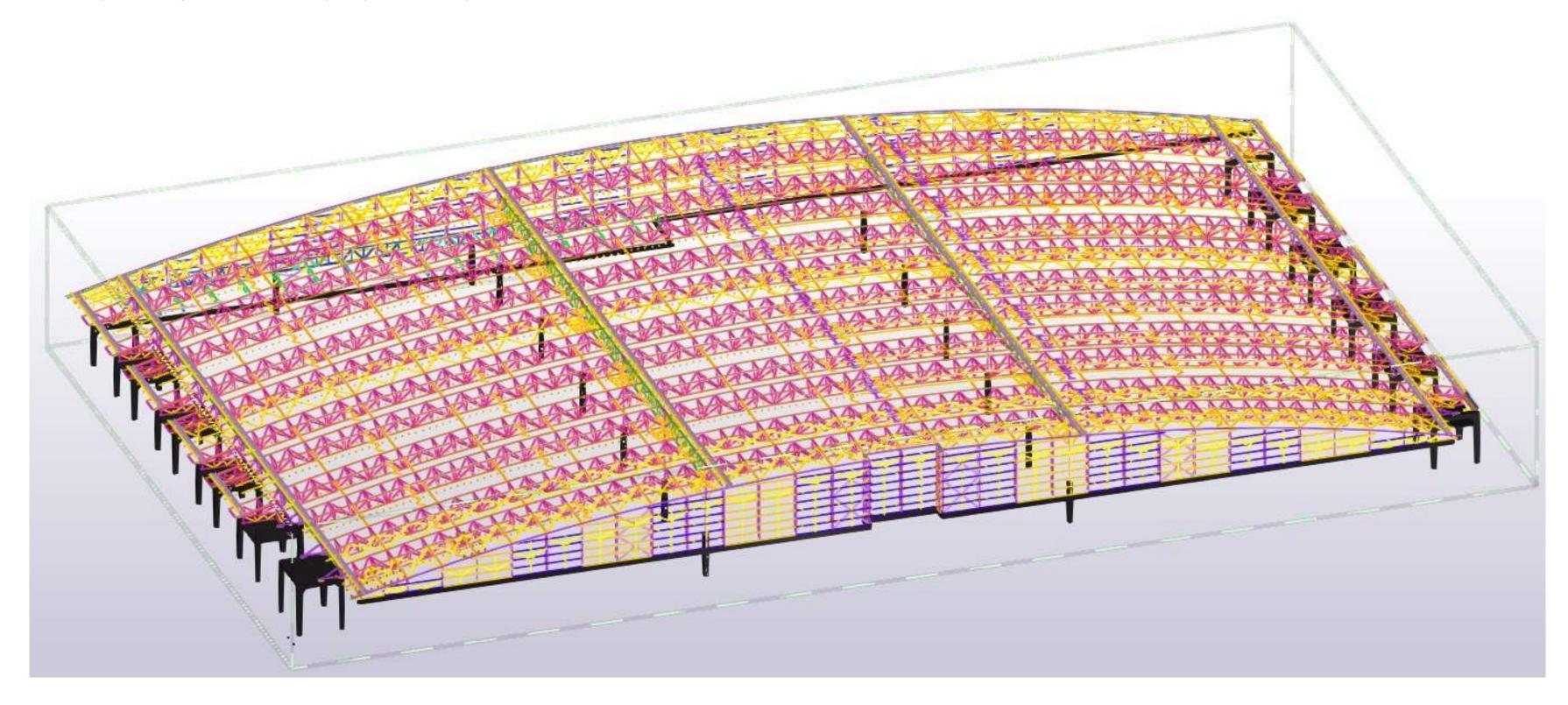
The idea of manufacturing 33 number similar toblerone trusses each being 70m. long and 3,6m. in size made up of piece small components required some innovative thinking with respect to how one would make suitable jigs to ensure that all the components would fit together correctly when it came to assembling them on site.
