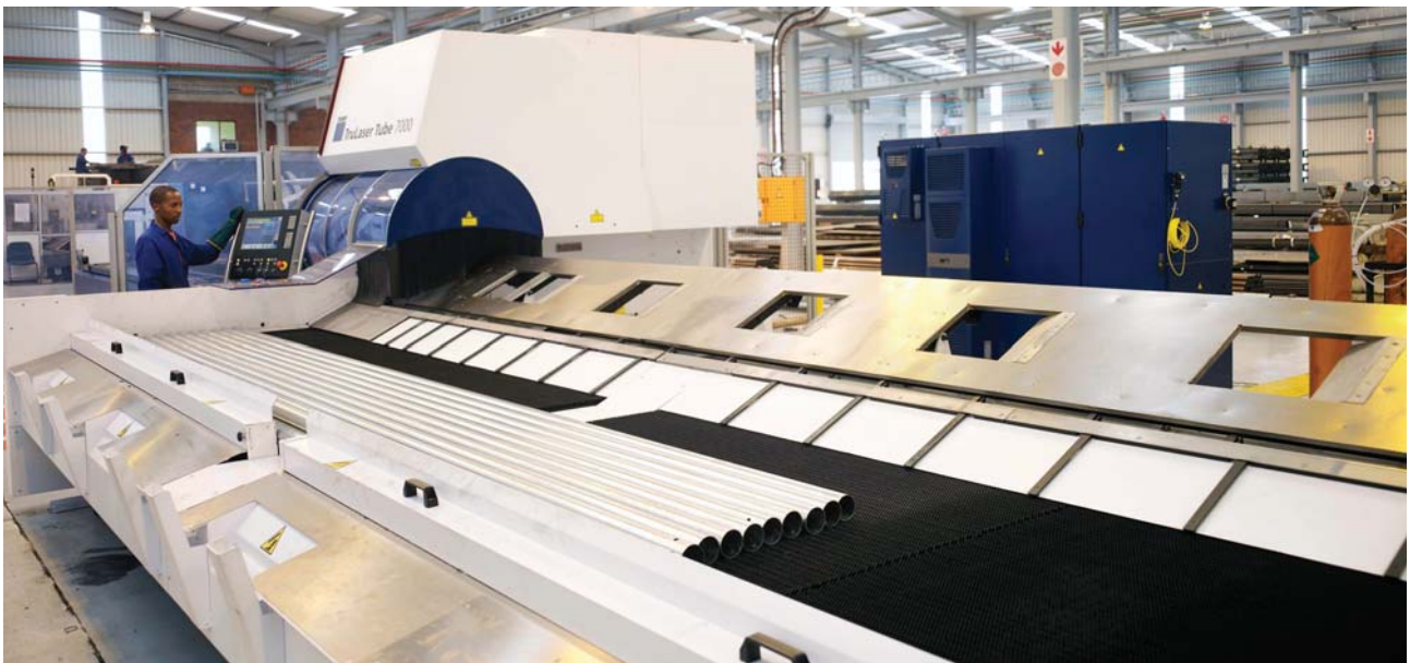
The Trumpf TruLaser Tube 7000 laser cutting machine is the first of its kind in South Africa
