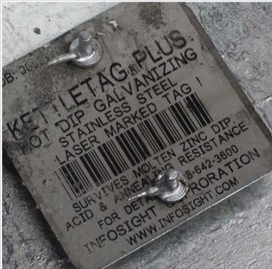
KettleTag® PLUS after galvanizing.
