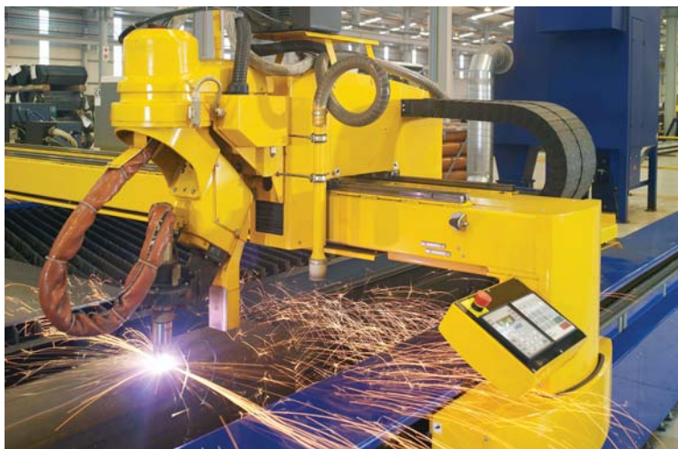
The Microstep HD Plasma Cutter is ideal for providing tube for structural applications and features a three dimensional head.
