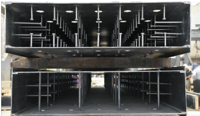
Modular composite shear wall that does not require climbing formwork.
