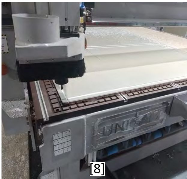
Fabrication of aluminium composite panels for exposed ceiling closure
